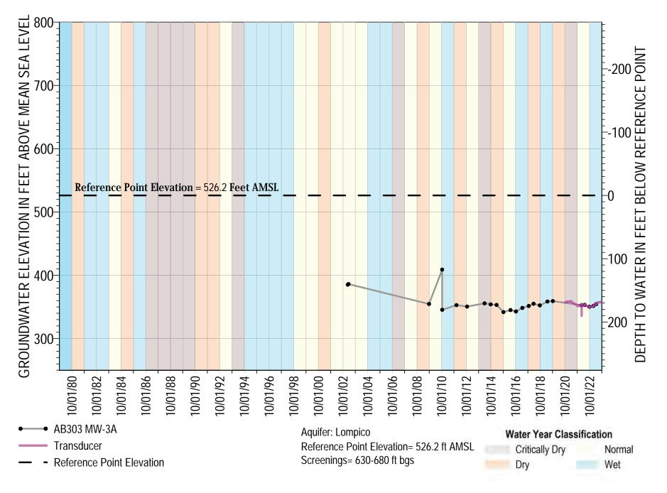
Note: Reference point is the elevation from which depth to water is measured at a well, typically 1-2 feet above land surface.
