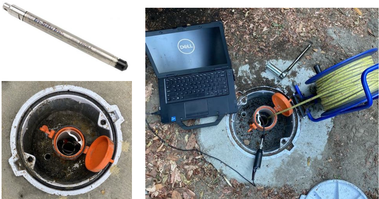
Figure 13. Example Transducer Equipping and Programming
