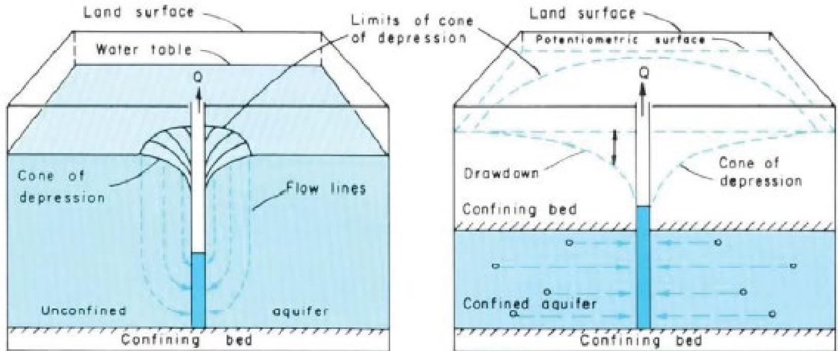
Figure 15. Cone of Depression Resulting from Well Pumping (Heath, 1983)
