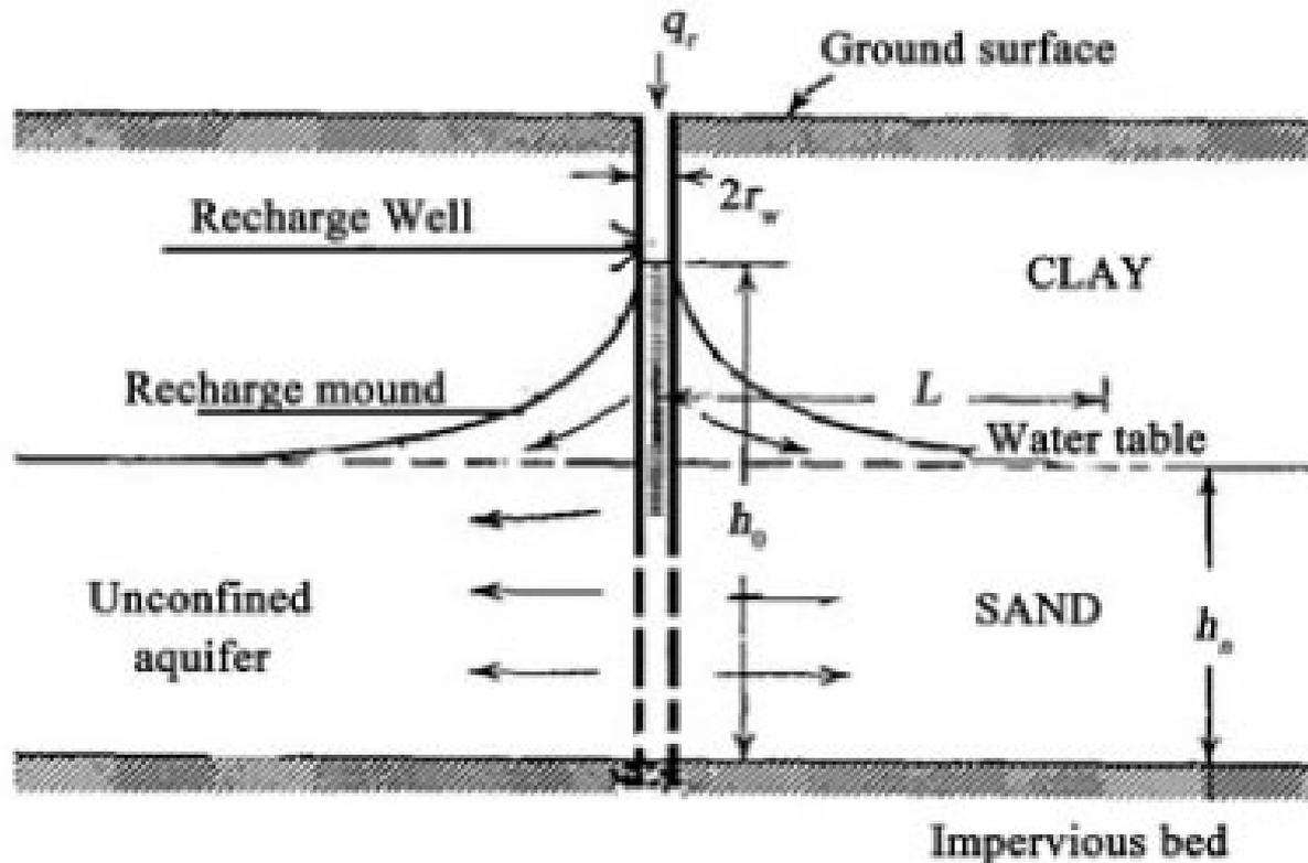
Figure 16. Groundwater Mound During Well Injection
