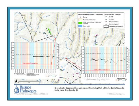
To use groundwater elevation as a proxy we need to show that there is a correlation between groundwater level and interconnected streamflow. We can look at groundwater levels from existing monitoring wells and compare the groundwater elevation to the elevation of a nearby streambed or GDE. If the groundwater level is higher than the streambed, then groundwater is contributing to streamflow. Changes in groundwater elevation will directly relate to groundwater contribution to streams.
