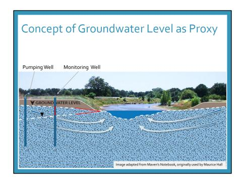
To use groundwater level as a proxy, we ideally want to have the monitoring well in between a pumping well and a GDE. We can then monitor the changes in the groundwater level. As the gradient of flow towards the GDE changes the groundwater contribution to GDEs changes.
