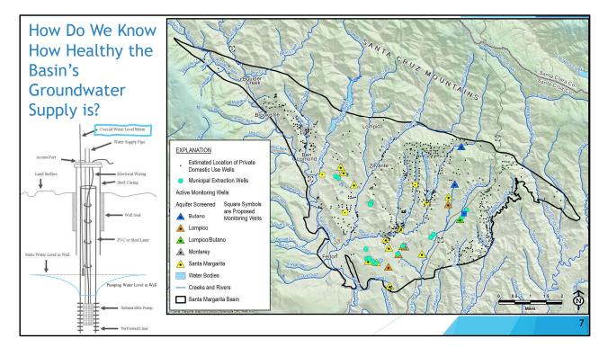
Map of where there are wells monitoring groundwater levels in the Basin. They are either public water supply wells themselves or monitoring wells that SLVWD and SVWD have installed to better manage the groundwater resources. The different colors indicate which aquifer the well monitors.
